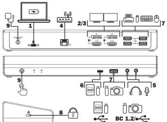
Connect the host computer or laptop to the U442-DOCK21-B using the included USB-C to C cable. Use the USB-A to C adapter if necessary.
