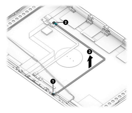
22. If you need to remove the second ambient light sensor cables, disconnect the cable from the ZIF connectors on the second ambient light sensor (1) and hub board (2), and then peel the cables off the inside of the display back cover to remove them (3).
