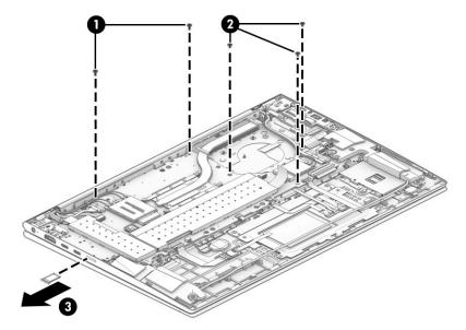
5. Lift the side of the system board upward (1), and then pull the system board away from the connectors on the side of the computer to remove it (2).
