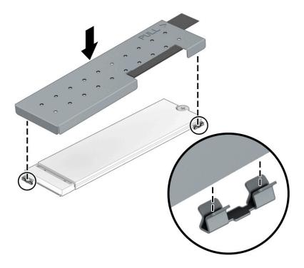
To install the solid-state drive, reverse the removal procedures.
