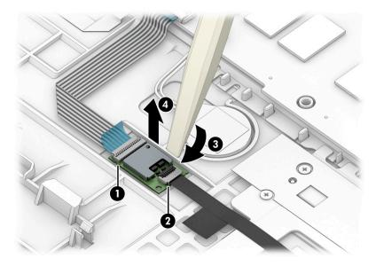
Reverse this procedure to install the NFC module.
