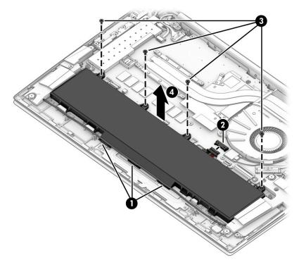
To insert the battery, reverse the removal procedures.
