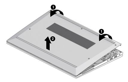
To replace the bottom cover, reverse the removal procedures.
