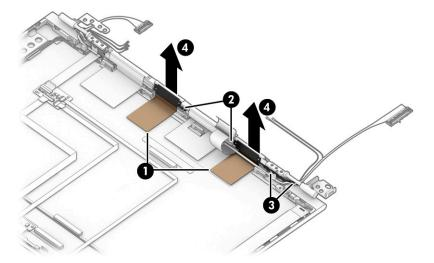
20. If you need to remove the WWAN antenna cables, peel the antennas off the inside of the display back cover (1), remove the cables from the clips in the back (2) and near the hinge on the display back cover (3), and then remove the antennas and cables (4).
