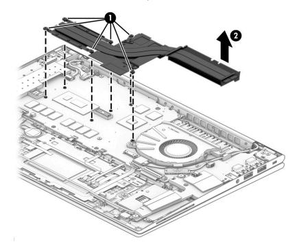
c. Thoroughly clean the thermal material from the surfaces of the heat sink and the system board components each time the heat sink is removed. Replacement thermal material is included with the heat sink and system board spare part kits. The following illustration shows the replacement thermal material locations.
