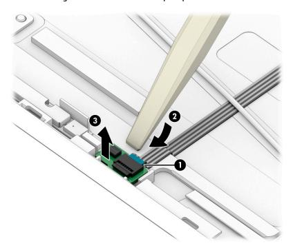
**14.** If you need to remove the second ambient light sensor from the display, disconnect the cables from the ZIF connectors on the board **(1)**, and then remove the sensor from the computer **(2)**.
