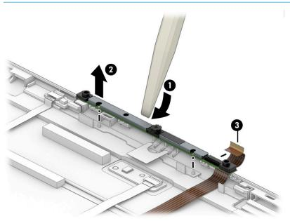
17. If you need to remove the display cable, disconnect the cable from the ZIF connector on the hub board (1), remove the cable from the clips at the bottom of the display back cover (2), and then remove the cable (3).
