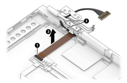
**18.** If you need to remove the camera cable, disconnect the cable from the ZIF connector on the hub board **(1)**, and then peel the cable off the inside of the display back cover to remove it **(2)**.
