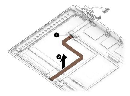
19. If you need to remove the WLAN antenna cables, peel the antennas off the inside of the display back cover (1), remove the cables from the clips at the bottom of the cover (2), (3), and then remove the antennas and cables (4).
