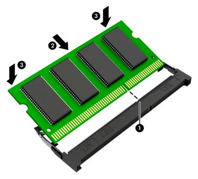
3. Replace the cover by inserting the edges of the cover into the clips on the system board that surround the memory modules (1).
