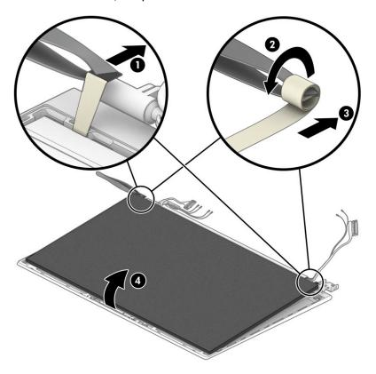
c. Lift the tape from the connector on the display panel (1), rotate the locking lever (2), and then disconnect the cable from the panel (3).
