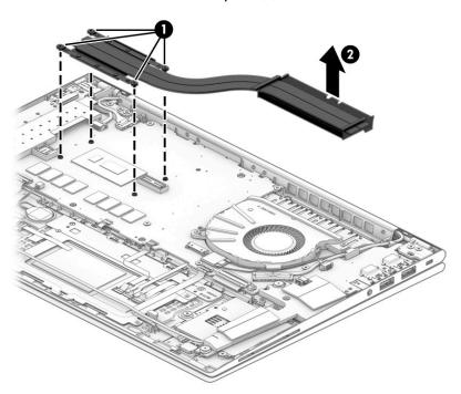
c. Thoroughly clean the thermal material from the surfaces of the heat sink and the system board components each time the heat sink is removed. Replacement thermal material is included with the heat sink and system board spare part kits. The following illustration shows the replacement thermal material locations.
