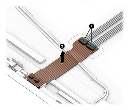
**15.** If you need to remove the microphone board from the display, disconnect the cable from the reverse ZIF connector on the board **(1)**, and then use a tool **(2)** to release the board from the computer **(3)**.
