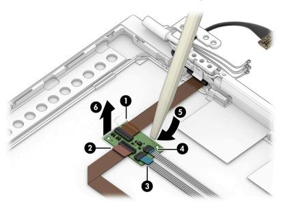
13. If you need to remove the ambient light sensor from the display, disconnect the cable from the reverse ZIF connector on the board (1), and then use a tool (2) to release the sensor from the computer (3).
