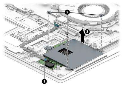
Reverse this procedure to install the card reader board.
