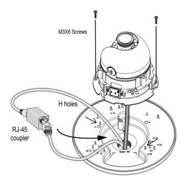
Note that for cameras that come with cable glands, e.g., FD8134 and FD8134V, it can be tricky passing them through a 3/4" pendant pipe.
