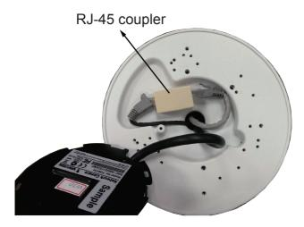
Align and install the camera to the bracket.
