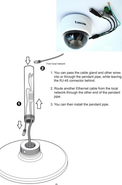
You can then connect the RJ-45 from the camera with that from the local network using an RJ-45 coupler. When done, press the coupler and the cables into the recess of the bracket.
