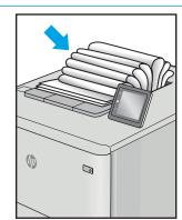
The paper does not stack well in the output tray. The stack might be uneven, skewed, or the pages might be pushed out of the tray and onto the floor. Any of the following conditions can cause this defect:
