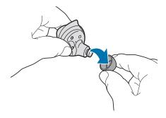
Do not pull the ear tip excessively when you attach or detach it. The ear tip may tear.
