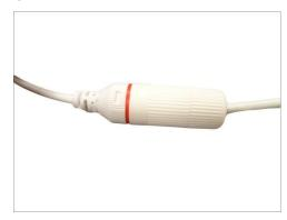
**NOTE:** Make sure the clamping nut is tightly attached to the cable gland body and the sealing insert is squeezed tightly.
