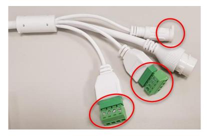
**NOTE:** If these connectors will not be used, make sure to wrap them with waterproof tape to avoid water or dust from entering the connectors.
