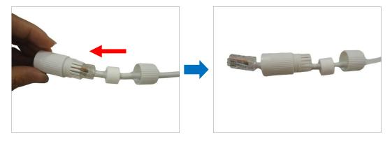
15. Push the sealing insert into the gland body.
