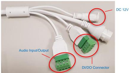
NOTE: If these connectors will not be used, make sure to wrap them with waterproof tape to avoid water or dust from entering the connectors.
