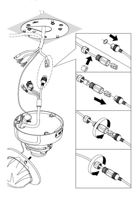
**NOTE:** If the camera will be installed outdoors or in places wherein environmental factors change drastically, make sure to waterproof the cable connections. See *How to Use the Cable Gland* on page 20.
