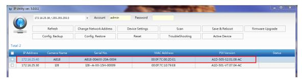
You can quickly see the camera model in the list. Double-click on the IP address to automatically launch the default browser of the PC with the IP address of the target camera filled in the address bar of the browser already.
