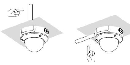
5. Mark the screw holes and cable hole (if the cable will pass through the surface) using the bundled surface mount plate as template. Then drill the necessary holes.
