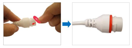
11. Detach the clamping nut and sealing insert from the gland body:
