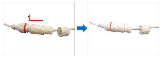
18. Attach the clamping nut to the gland body to complete the cable solution.
