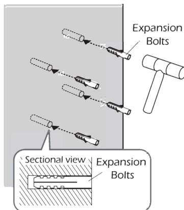
2. Knock the expansion bolts completely into the wall.
