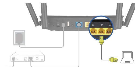
**Connect your PC** to the router via Wi-Fi or using an additional network cable (not included).
