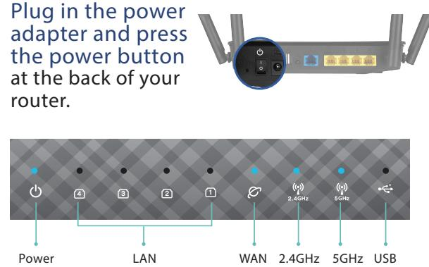
**Check the WAN and 2.4G / 5G LED lights** to ensure the hardware connection is ready (see the picture above).
