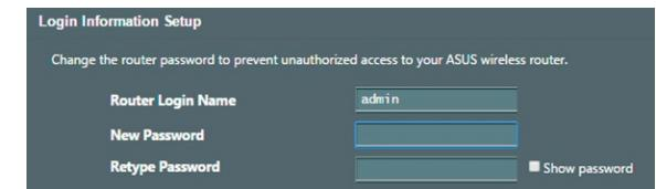
**Set up the router login information.** Assign unique login name and password for your router to prevent unauthorized access.
