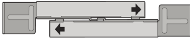
Figure 4: Bracket halves attachment procedure
