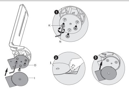
2b-1. Clamp Assembly for Desktops 0.6 - 1 in. (15 - 25 mm) Thickness
