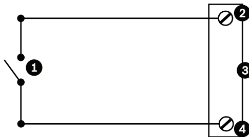
Figure 10.4: N.O. - Normally Open Non-supervised Connections
