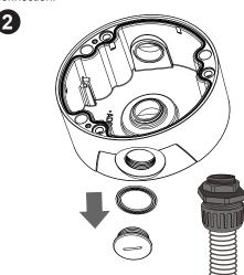
Install the cable gland and pass cables through it.
