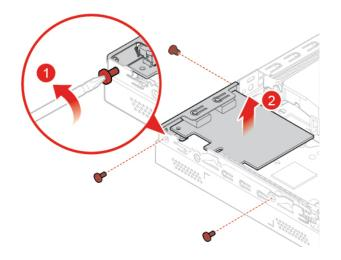
Figure 38. Removing the PCI Express card
