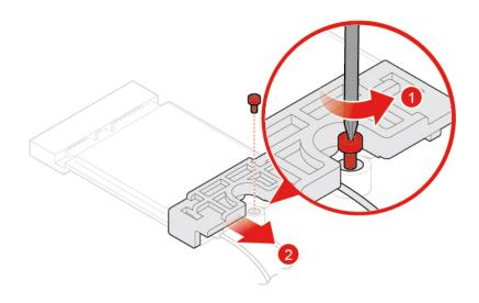
Figure 60. Removing the Wi-Fi card shield
