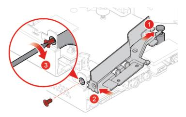
Figure 83. Installing the antenna bracket
