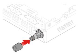
Figure 80. Installing the antenna cover to secure the rear Wi-Fi antenna cable
