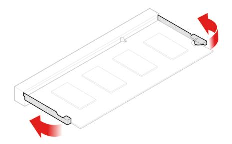
Figure 86. Opening the memory module retainer
