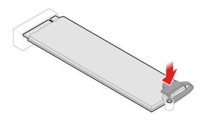
Figure 93. Locking the M.2 solid-state drive clip
