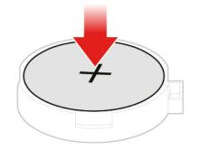
Figure 53. Pressing the coin-cell battery downward
