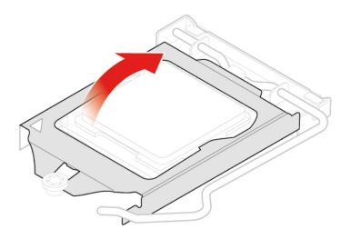
Figure 55. Pivoting the microprocessor socket upward
