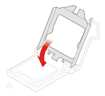
Figure 58. Pivoting the microprocessor socket downward
