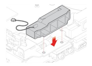
Figure 74. Installing the front Wi-Fi antenna
