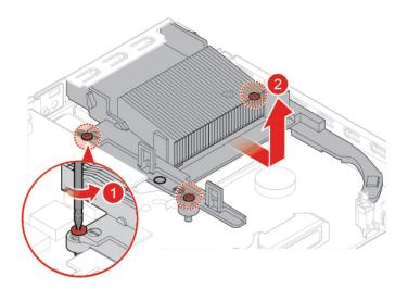
Figure 48. Removing the heat sink
