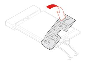
Figure 65. Installing the Wi-Fi card shield
