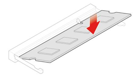
Figure 89. Closing the memory module retainer
