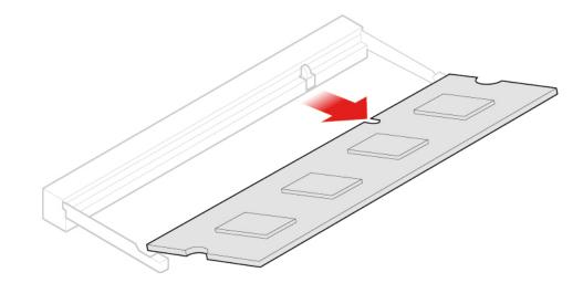
Figure 87. Removing the memory module
