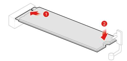
Figure 92. Installing the M.2 solid-state drive
