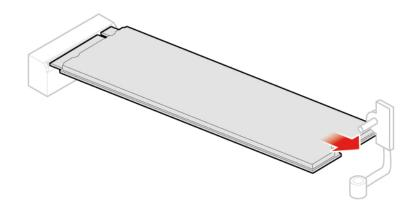
Figure 91. Removing the M.2 solid-state drive
