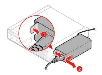
Figure 28. Removing the power adapter bracket
