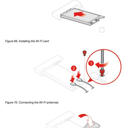
Figure 71. Installing the Wi-Fi card shield
