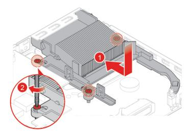
Figure 49. Installing the heat sink
