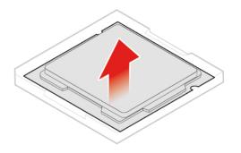
Figure 56. Removing the microprocessor
