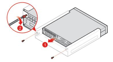
Figure 23. Installing the VESA mount bracket
