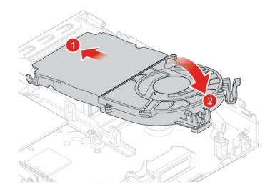
Figure 47. Installing the system fan
