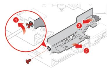
Figure 82. Removing the antenna bracket
