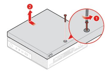
Figure 24. Removing the external optical drive box
