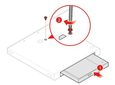
Figure 26. Installing the external optical drive
