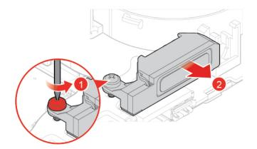
Figure 44. Removing the advanced speaker
