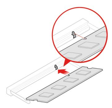
Figure 88. Installing the memory module
