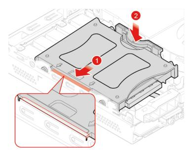
Figure 35. Installing the storage drive bracket
