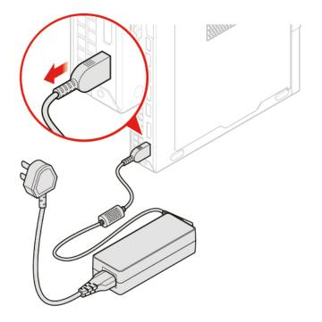
Figure 16. Removing the power adapter
