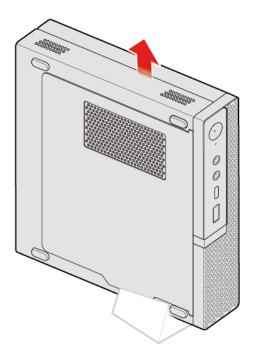
Figure 20. Removing the vertical stand
