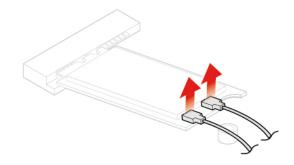
Figure 67. Disconnecting the Wi-Fi antennas
