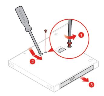
Figure 25. Removing the external optical drive
