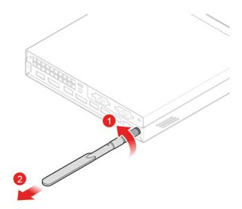
Figure 76. Removing the rear Wi-Fi antenna
