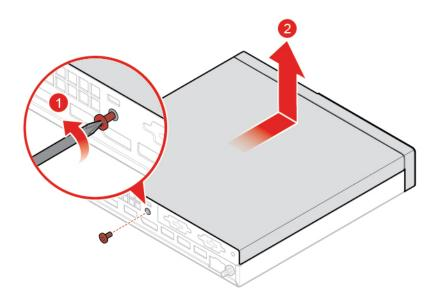
Figure 31. Removing the computer cover
