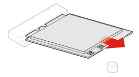
Figure 62. Removing the Wi-Fi card
