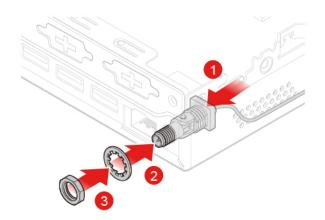
Figure 79. Installing the rear Wi-Fi antenna cable
