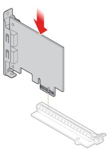
Figure 40. Installing the PCI Express card adapter
