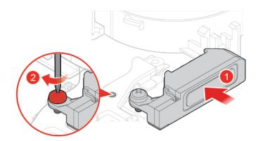
Figure 45. Installing the advanced speaker
