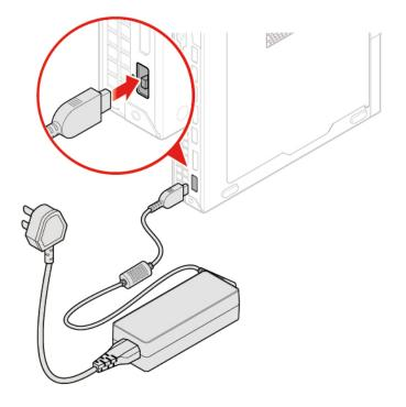
Figure 19. Installing the power adapter
