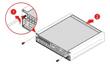
Figure 22. Removing the VESA mount bracket
