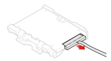
Figure 36. Removing the storage drive cable
