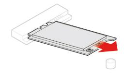
Figure 68. Removing the Wi-Fi card
