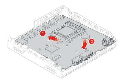
Figure 96. Installing the system board
