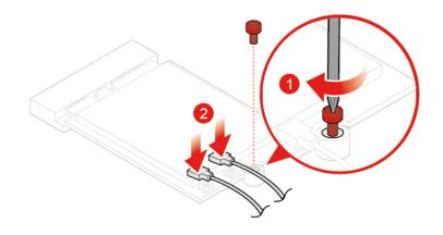
Figure 64. Connecting the Wi-Fi antennas
