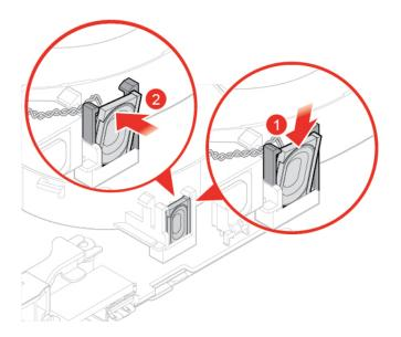
Figure 43. Installing the internal speaker
