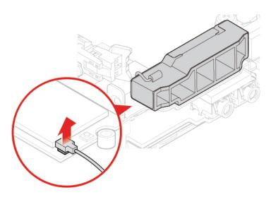
Figure 72. Disconnecting the front Wi-Fi antenna cable from the Wi-Fi card
