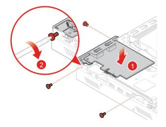
Figure 41. Installing the PCI Express card
