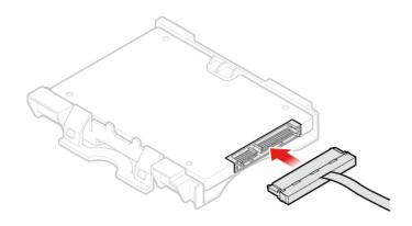
Figure 37. Installing the storage drive cable
