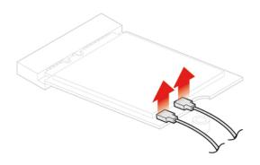
Figure 61. Disconnecting the Wi-Fi antennas
