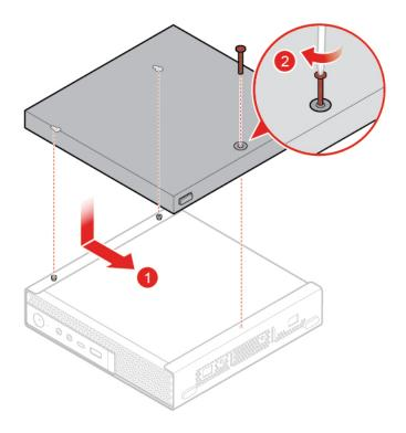
Figure 27. Installing the external optical drive box
