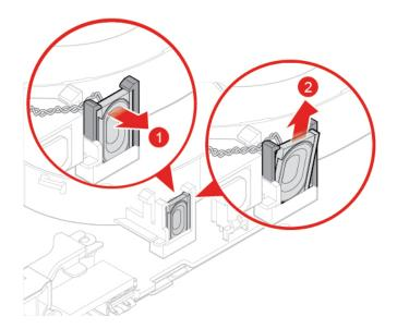
Figure 42. Removing the internal speaker
