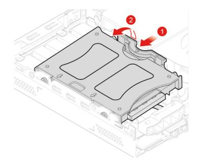
Figure 32. Removing the storage drive bracket
