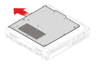
Figure 84. Removing the bottom cover
