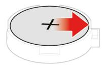
Figure 50. Pressing the metallic tab
