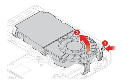
Figure 46. Removing the system fan
