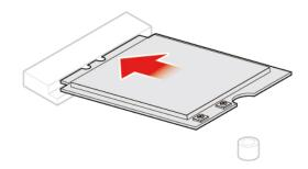
Figure 63. Installing the Wi-Fi card
