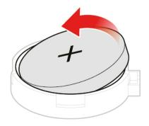
Figure 51. Removing the coin-cell battery
