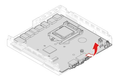
Figure 95. Removing the system board
