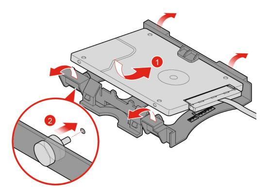
Figure 34. Installing the storage drive
