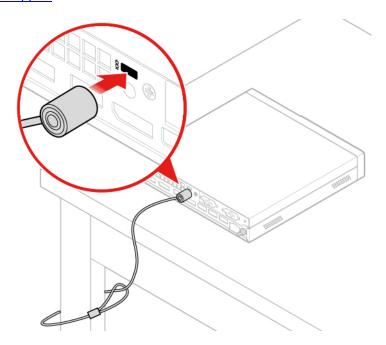
Figure 5. Attaching a Kensington-style cable lock
