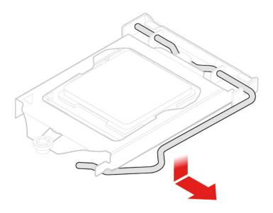
Figure 54. Unlocking the microprocessor socket retainer
