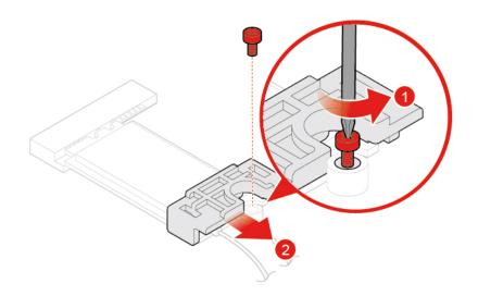
Figure 66. Removing the Wi-Fi card shield
