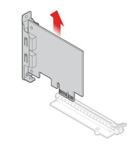
Figure 39. Removing the PCI Express card adapter
