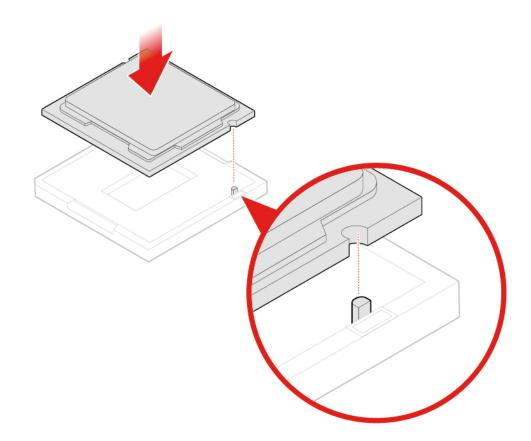
Figure 57. Installing the microprocessor
