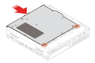
Figure 85. Installing the bottom cover
