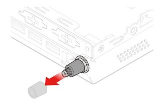
Figure 77. Removing the antenna cover that secures the rear Wi-Fi antenna cable
