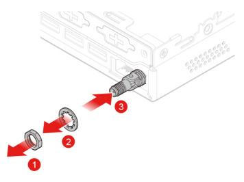
Figure 78. Removing the rear Wi-Fi antenna cable
