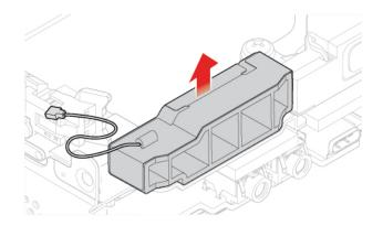
Figure 73. Removing the front Wi-Fi antenna
