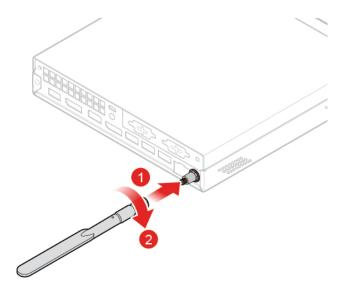
Figure 81. Installing the rear Wi-Fi antenna
