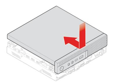
Figure 98. Reinstalling the computer cover
