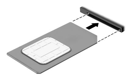
To remove a SIM card, press in on the SIM card, and then remove it from the slot.
