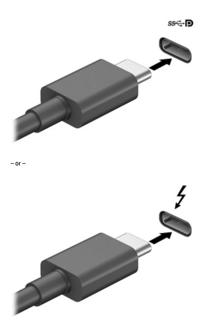
2. Connect the other end of the cable to the external device.
