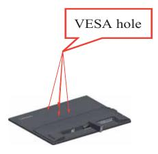
Step 5: Attach the LCD display to the wall, and follow the instructions in the wall-mounting kit.
