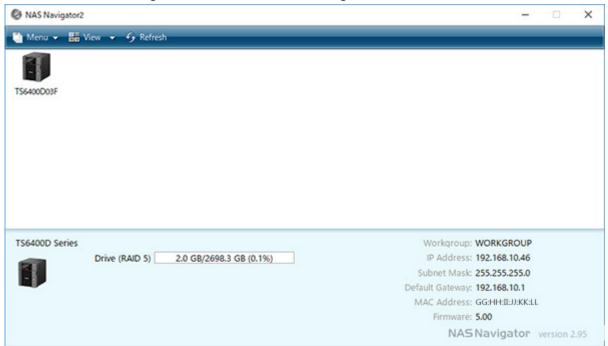
Click a Buffalo NAS device's icon to display total capacity, used space, workgroup name, IP address, subnet mask, default gateway, MAC address, and firmware version.
