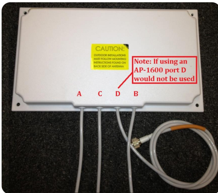
Figure 44. Patch antenna leads
