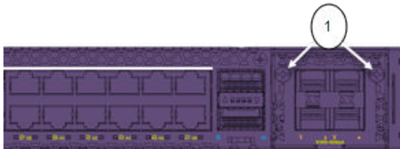
Figure 19: Tighten Screws on the Inserted VIM5 Module
