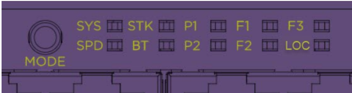
Figure 26: VSP 4900 Mode and System Status LEDs
