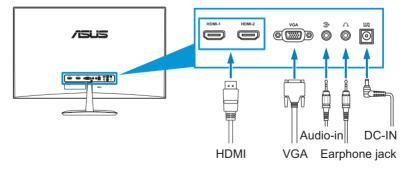
To connect the audio cable: connect one end of the audio cable to the monitor's Audio-in port, the other end to the computer's audio-out port.
