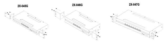
**2.** Screw the mounting brackets to the rack to complete the installation.
