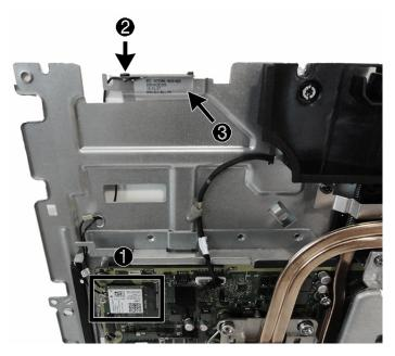
12. Remove the Phillips screw from the left antenna (1), and then peel the antenna from the chassis (2).
