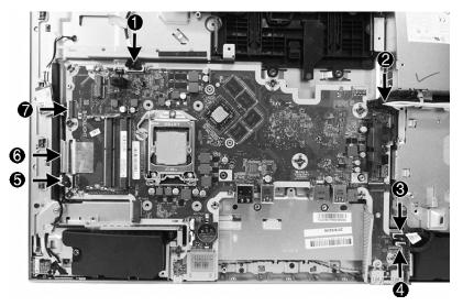
**15.** In the order printed on the system board, remove the nine Torx screws **(1)-(9)** that secure the system board to the computer.
