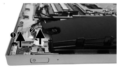
**7.** If necessary, disconnect the cables from each board.
