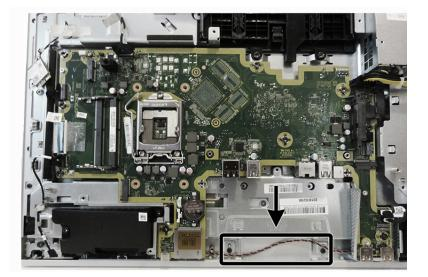
To remove the RFID board:
