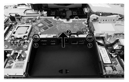
To install the bottom I/O cover, reverse the removal procedures.
