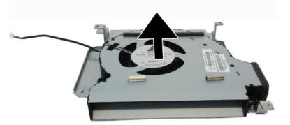
To replace the VESA mounting bracket/fan assembly, reverse the removal procedures.
