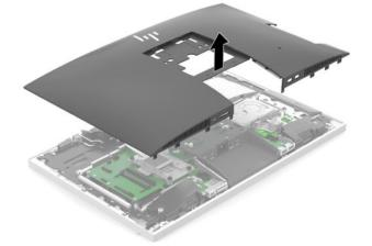
To replace the access panel, reverse the removal procedures.
