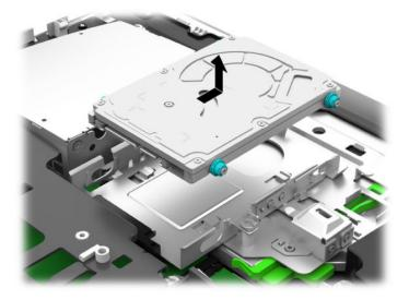
7. Remove the four mounting screws from the 2.5-inch hard drive. Be sure to keep the screws together with the blue rubber grommets to use to install a replacement drive.
