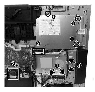
**10.** Remove the power supply from the computer.
