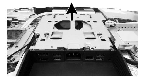
8. If it is necessary to remove the fan from the bracket, remove the four Torx screws that secure the fan to the bracket.
