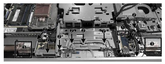
To install the RF asset module antennas, reverse the removal procedures.
