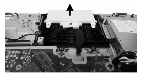
If you need to remove the webcam bracket, remove the VESA bracket/fan assembly (<u>VESA mounting bracket/fan assembly on page 48</u>), and then remove the four Torx screws (1) that secure the webcam bracket to the computer.
