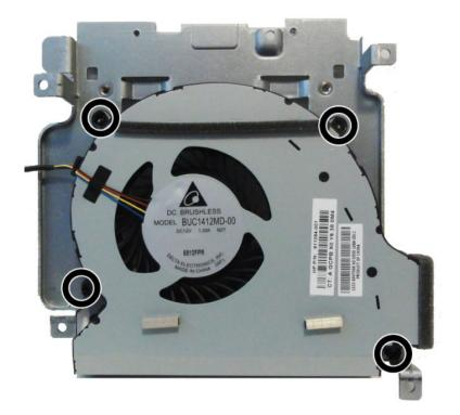
**9.** Separate the fan from the bracket.
