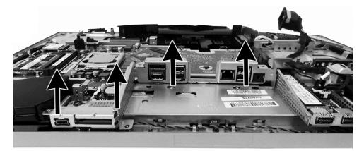
To replace the I/O bracket, reverse the removal procedures.
