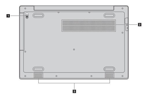
Optical disk drive/ removable battery latch (on select models) The spring-loaded latch keeps the optical disk drive/removable battery secured in place.
