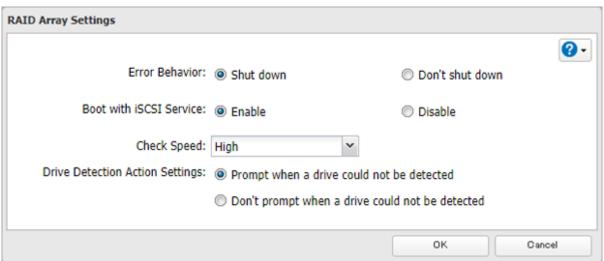
When the confirmation screen is hidden, an undetected drive will automatically be dismounted from the TeraStation and the TeraStation will be in degraded mode if a redundant RAID mode is configured. If RAID 0 is configured, the
