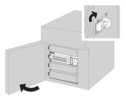
$oldsymbol{2}$  The failed drive's status LED will be glowing red. Push its unlock button and swing the lock mechanism out.
