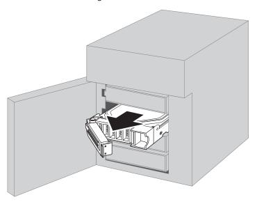
**4** Insert the new drive into the empty slot. Slide the drive in with the locking mechanism open.
