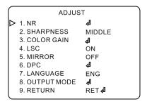
**NR** (**Noise Reduction**): You can adjust the camera's digital noise reduction settings to 2DNR and 3DNR. Digital noise reduction helps decrease digital noise in low lightning and make the image more thorough. Increasing the value of the digital noise reduction will make improve the digital noise reduction effect but it may also reduce the image resolution.
