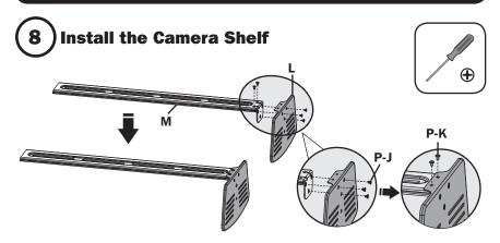
Using M4x6 screws (P-J) and (P-K), attach the camera shelf to the connecting plate.
