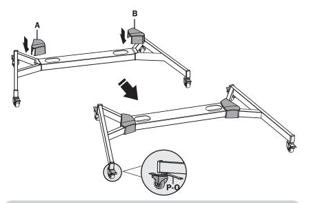
**Note:** Lock the brakes on the casters to avoid any sudden movements during installation. Each caster can be adjusted independently for fine adjustments. Slightly turn each caster nut to lower or raise the base.
