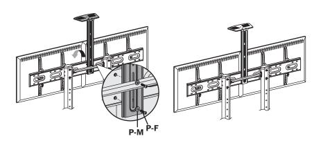
Using M6x25 screws (P-F) and D6 washers (P-M), attach the connecting plate to the universal plate.
