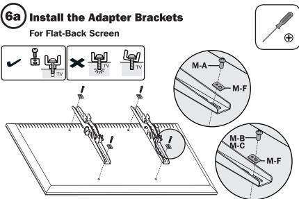
Note: Choose appropriate screws and washers according to the type of screen.
