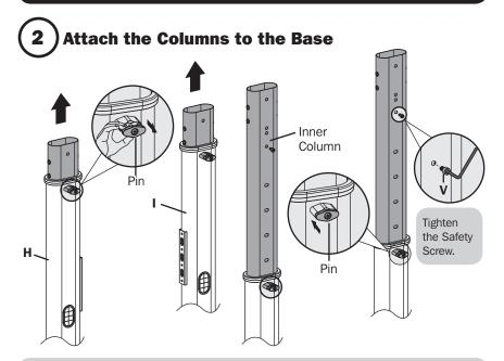
Pull the pin outward and lift the inner column upward at the same time until the inner column is at the desired height. Release the pin to secure.
