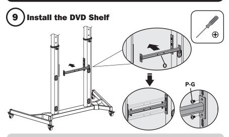
Using M6x8 screws (**P-G**), attach the support bar to the columns at the desired position.
