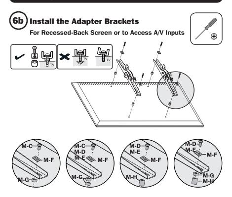
**Note:** Choose appropriate screws, washers and spacers (if necessary) according to the type of screen.
