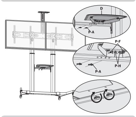
Using M6x25 screws (**P-F**), M6x8 screws (**P-H**) and butterfly nuts (**P-A**), attach the DVD shelf to the support bar.
