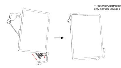
3b. Insert tablet corner against the spring arm. Push adjustable arm down against opposite corner (A). Be sure it is as snug as possible. Be sure to not place on the corner where camera would be on tablet or else it will block.
