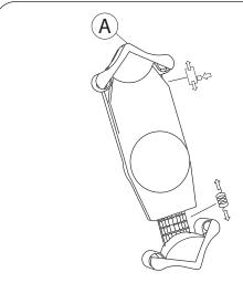
3a. Press quick release button on side of tablet holder (A) to release the adjustable end.
