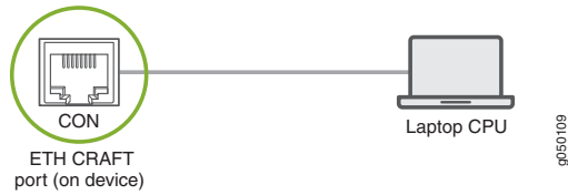
Figure 24: Connecting the ACX6160 Directly to a Management Console
