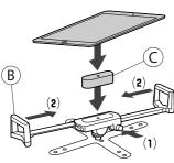
2B. Insert the tablet in Security Universal Holder (B) with the correct foam pad (C). Identify the right foam pad by testing your tablet with various pieces until you find the one that fits securely and snug.
