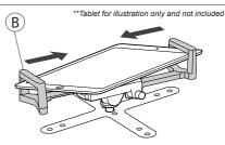
2C. Insert the tablet then retract the arms until the tablet and holder fits securely.
