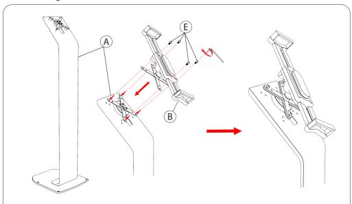
security holder (B) to the threaded VESA 100mm X 100mm holes until securely tightened.
