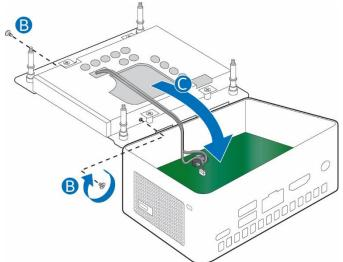
4. Secure the drive into the drive bay with the four screws that were used in step 1. Set the drive bay bracket down inside the chassis (C).
