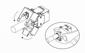
5. Fasten the cable tie around the cable fixture to secure the cable to the keystone jack.
