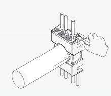
3. Insert the cable into the termination cap and fan out all four twisted pairs. Using the T568A or T568B color labeling, position each wire appropriately into the color labeled slots. Cut excess wires.
