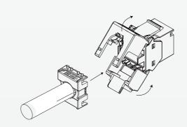
4. Secure the hinged panels using a crimping tool until they are firmly snapped together.
