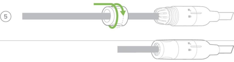
3a. If using conduit adapter, attach the terminal adapter to the conduit adapter. Route the conduit over the water-tight cable gland assembly and terminate at the terminal adapter. Ensure the camera conduit adapter is securely placed on the base mount plate as pictured.
