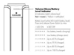
NOTE: When operating on battery, unit will power down automatically after 15 minutes of no audio unless connected to Wi-Fi.
