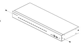
Use the M3 x 8 Phillips hex head screws supplied with the rack mounting kit to screw the rack mounting brackets into the sides near the front of the switch
