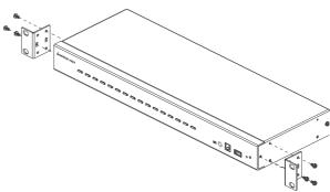
Place the KVM switch into the rack. Position the switch so that the holes in the mounting brackets line up with the holes in the rack. Secure the mounting brackets to the front of the rack
