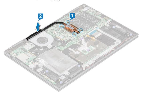
NOTE: Loosen the captive screws using a diagonal or crisscross pattern as printed on Heatsink. The screws are captive screws and cannot be fully removed.
