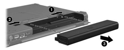
Removing the Battery Pack
