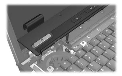
Removing the Switch Cover
