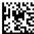
GS1 DataBar Expanded GS1-128 Emulation = Enable
