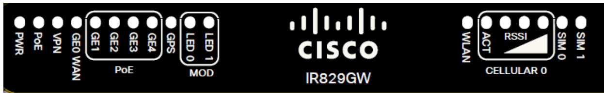
Figure 1-6 Cisco IR829 LED Detail
