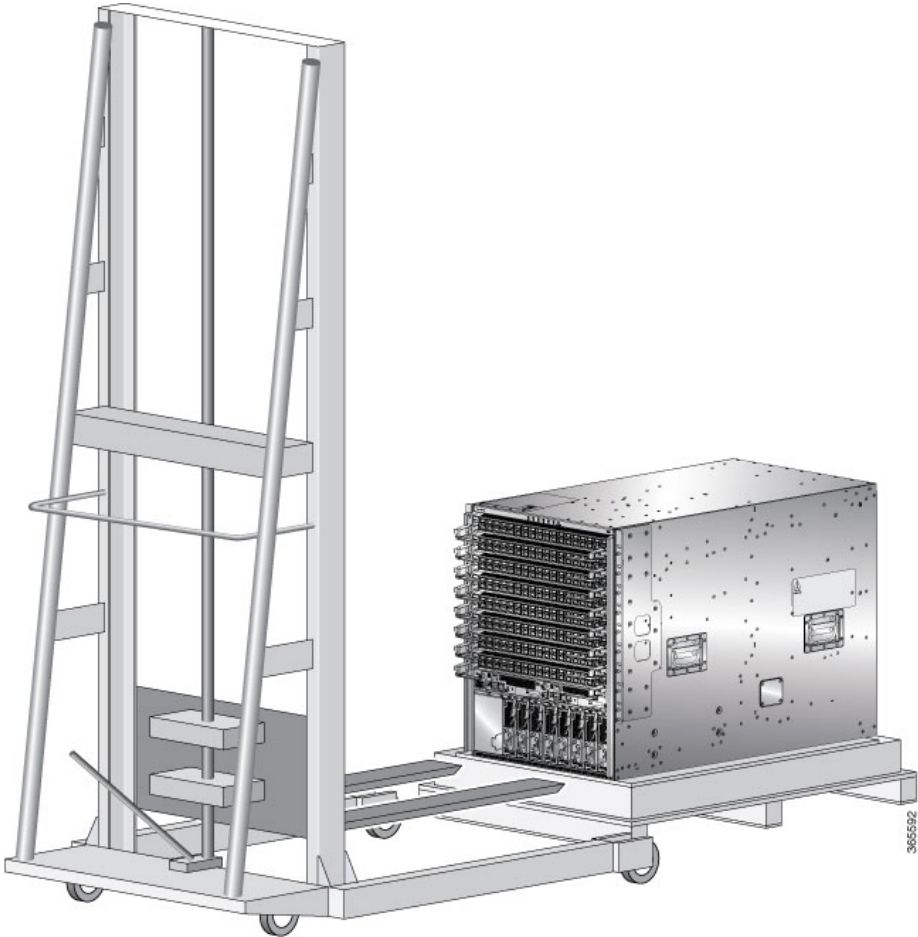
Figure 22: Align the Lifting Device In Front of the Chassis on the Pallet
