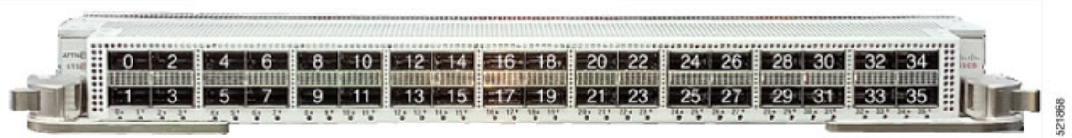
Figure 8: Port Numbering on NC57-36H6D-S Line Card
