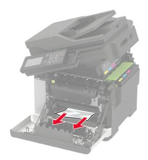
${\bf 3}~$  Open the fuser access door, and then remove the jammed paper.
