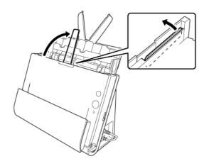
4 Set the feed selection lever and the eject selection lever.
