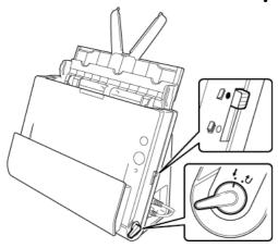
2 Adjust the document guides to fit the width of the card to be scanned.
