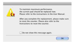
If this message begins to be displayed at startup, purchase an exchange roller kit and replace the worn parts with the consumable parts included in the kit (feed roller and retard roller). For details on the exchange roller kit, see "Exchange roller kit (product code: 5484B001)" on p.111.
