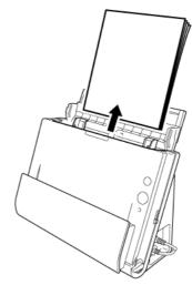
2 When the jammed document is on the document ejecting side, open the document eject tray.
