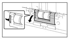
2 Remove the retard roller and then install the new retard roller. When installing the retard roller, align the notch on the roller with the shaft of the main unit.
