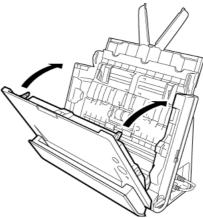
After removing the jammed paper, check to see if the last page was scanned correctly, and then continue scanning.
