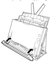
5 Press the OPEN button and pull open the front unit toward you.
