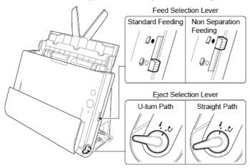
The feed and eject methods and lever positions for each document type are as follows.
