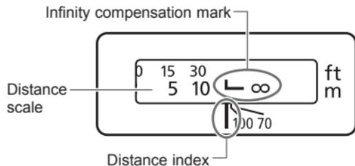
To compensate for shifting of the infinity focus point that results from changes in temperature, there is a margin at the infinity ( $\infty$ ) position. The infinity position at normal temperature is the point at which the vertical line of the distance scale L mark is aligned with the distance index.
