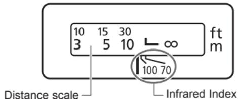
The infrared index corrects the focus setting when using monochrome infrared film. Focus on the subject manually, then adjust the distance scale indicated by the distance index by moving the focusing ring to the corresponding infrared index mark before shooting.
