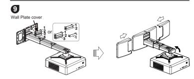
Note: When all adjustments are done, the wall plate covers can be used to cover the blank area on the top of wall plate. The number of wall plate cover used depends on the size of blank area. But the wall cover must be used in an specific order as the picture on left shows. Finally, put the wall cover on.
