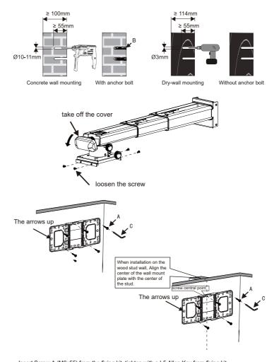
• Insert Screw A (M6x55) from the fixing kit, tighten with a L5 Allen Key from fixing kit.
