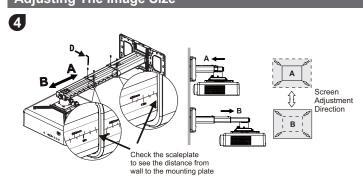
Note: To make adjustments to meet your demands, screws must be loosened in a specific order, as shown in the above figure. (When the length of inside arm 895mm do not meet your demands, then you should loose the screws on the outside arm to adjust the middle arm. Under this circumstance, the number read on the middle arm is correct).
