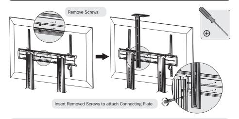
Remove the Universal Plate's two rear screws, then attach the Camera Shelf Assembly using the same screws just removed. Adjust the Camera Shelf Assembly to the desired height, then secure by tightening the screws with a Philips screwdriver.
