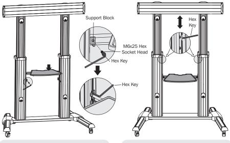
Use the Hex Key and screws to secure the DVD Shelf Assembly to the Columns' Support Blocks.
