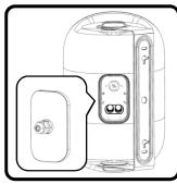
6. Tightly insert terminal cover into the cabinet groove
