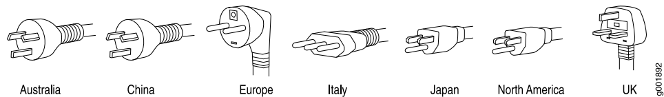
Figure 5: AC Plug Types
