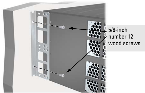
Figure 2-12. Mounting to a wall
