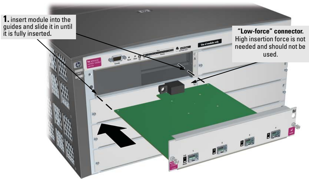
Figure 2-1. Installing a module
