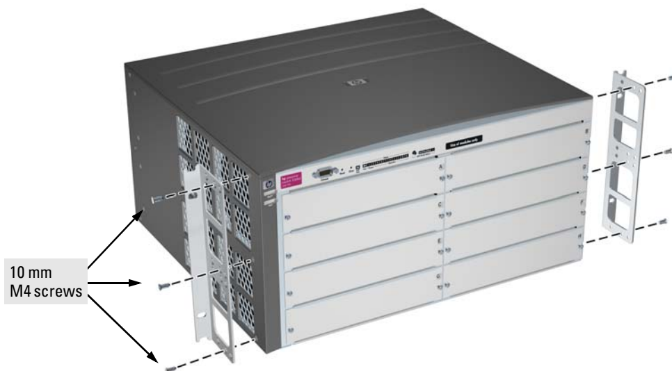
Figure 2-7. Attaching brackets to the switch 5308xl
