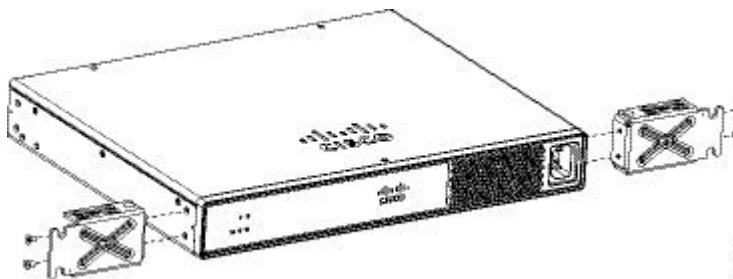
Figure 6: Bracket Installation for Back Mounting
