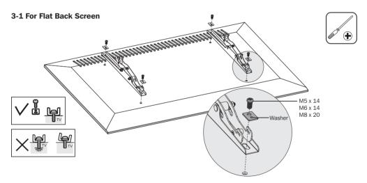
Note: Choose appropriate screws, washers and spacers (if necessary) according to the type of screen.
