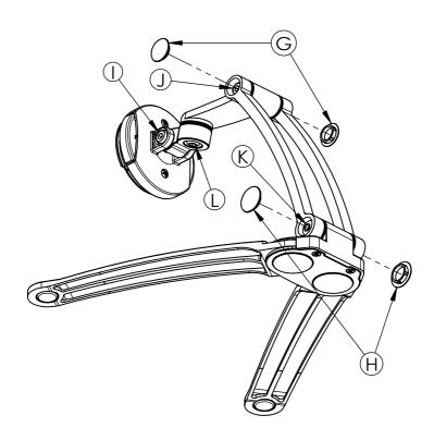
XPlease adjust the tightness of the joints when they are loose after use for a while.
