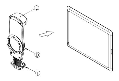
Attachment Description 1 : Press D and stretch F till larger than the length of tablet. Then release D .
