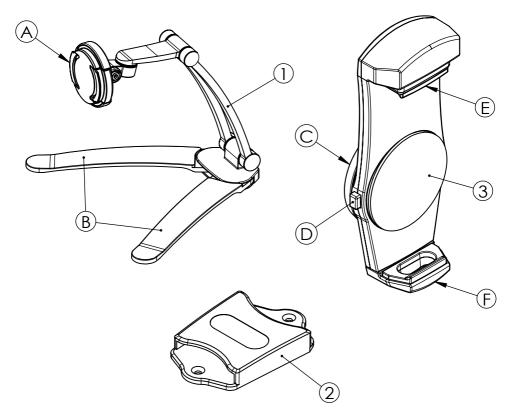
\*\*Note - Hinges may get looser and droop over time. Please tighten screws for optimum usage and efficiency.
