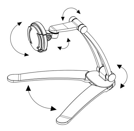
\*\*Note - Hinges may get looser and droop over time. Please tighten screws for optimum usage and efficiency.
