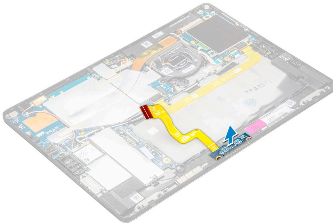
Lift the docking board after releasing the cable from the adhesive.
