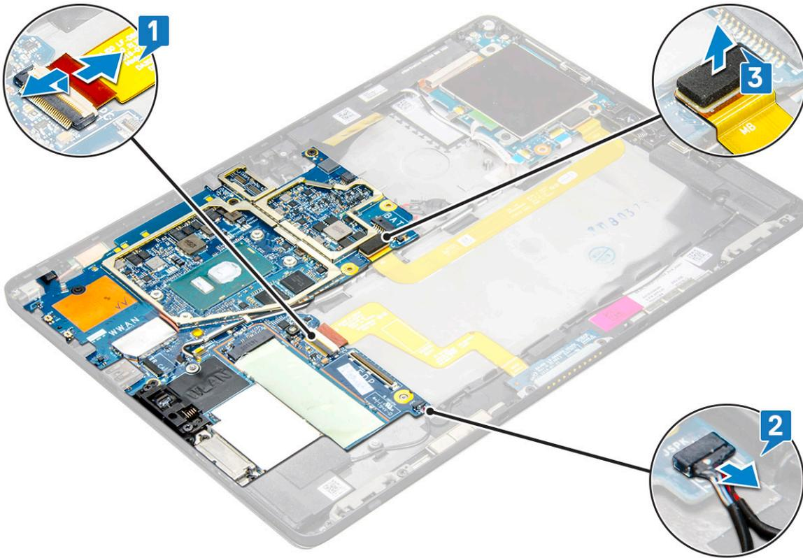
4 Un route the antenna cables from the routing clips [1,2,3].
