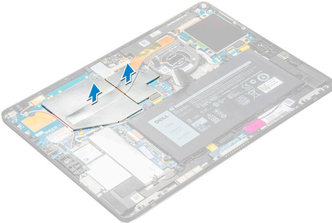
4 To remove the heat sink assembly:
